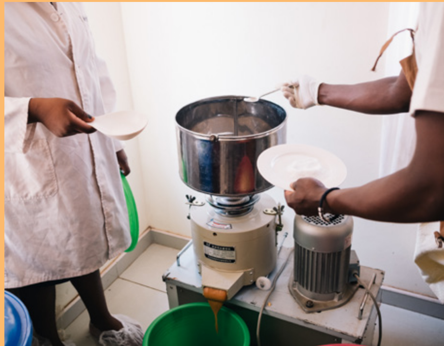
This machine is used to grind peanuts and turn them into butter.
